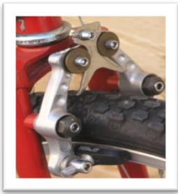
Every bike must have a way to stop. Brakes on a bike work because of friction. Many bikes have brakes that are **activated** by squeezing a rubber shoe against the rim of the wheel causing the wheel rotation to slow. As the brake shoe is rubbing against the wheel rim, your kinetic energy is converted into heat, which has the effect of slowing you down.
