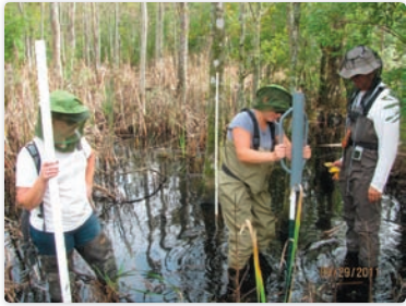
NCSU scientists and park staff install water level gauges at Goose Creek State Park to determine the degree to which a park road may be influencing vegetation changes.
